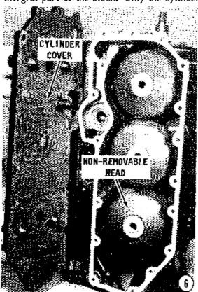
cover is removable to provide access to the water jacket for cleaning and inspecting purposes.
