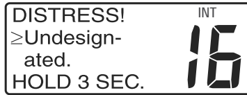
Distress Alert Screen
